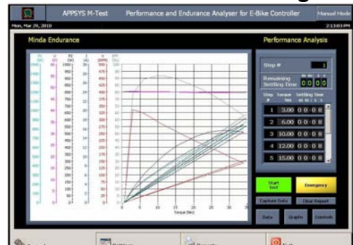
E Bike-BLDC Motor Testing
