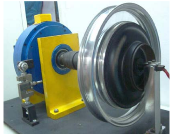
E Bike-BLDC Motor Testing
