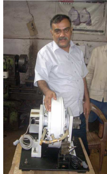
150 Nm Water cooled Powder Dynamometer
