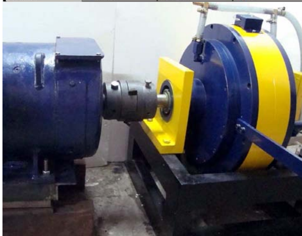
POWDER DYNAMOMETER used for Motor & Wiper Motor Testing
